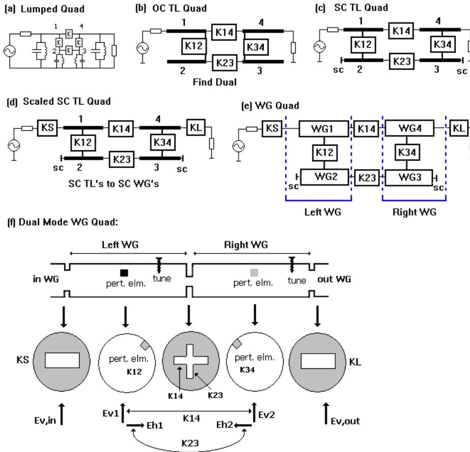
Fig. 2. Dual mode waveguide quadruplet design stages.
