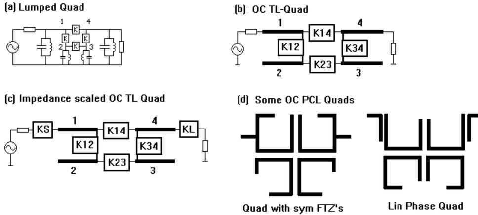
Fig. 1. Microstrip type parallel coupled line quadruplet design stages.
